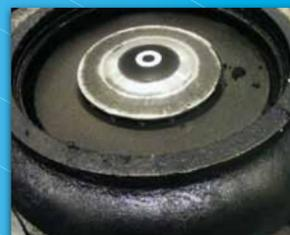
Compressor end oil leakage
