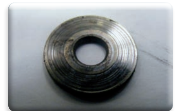
This marking is evidence of contaminated oil
