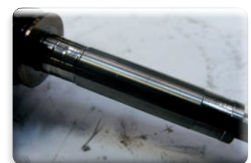
Extreme wear on the turbine shaft
