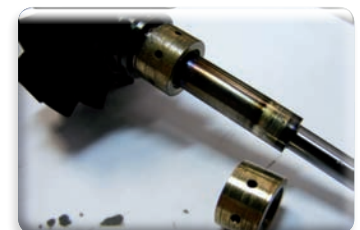
The blue colouring indicates excessive temperatures
