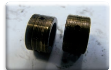
Severe scoring on to the journal bearings
