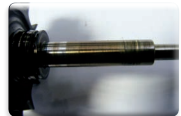
Extreme heat damage due to lack of oil
